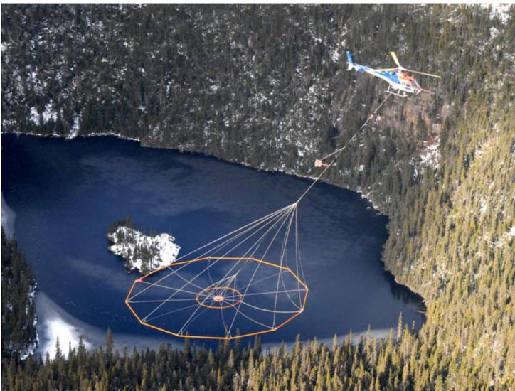
*Aerial Electromagnetic Survey. Photo: Geotech,
